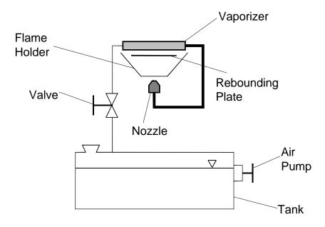
**Figure 1:** Function diagram of a pressure stove
